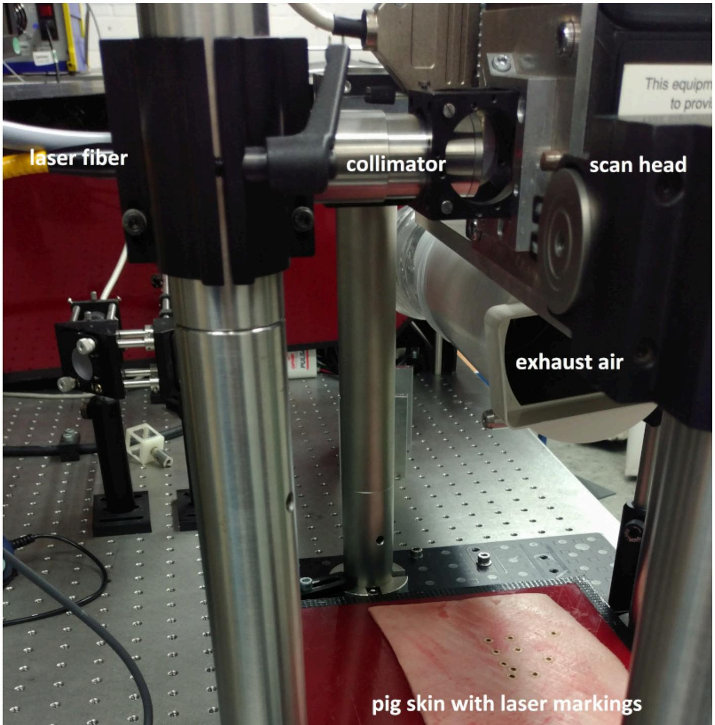
Figure 2: The laboratory setup to find out the best parameters for robust laser markings. Source: M. Geggus.
